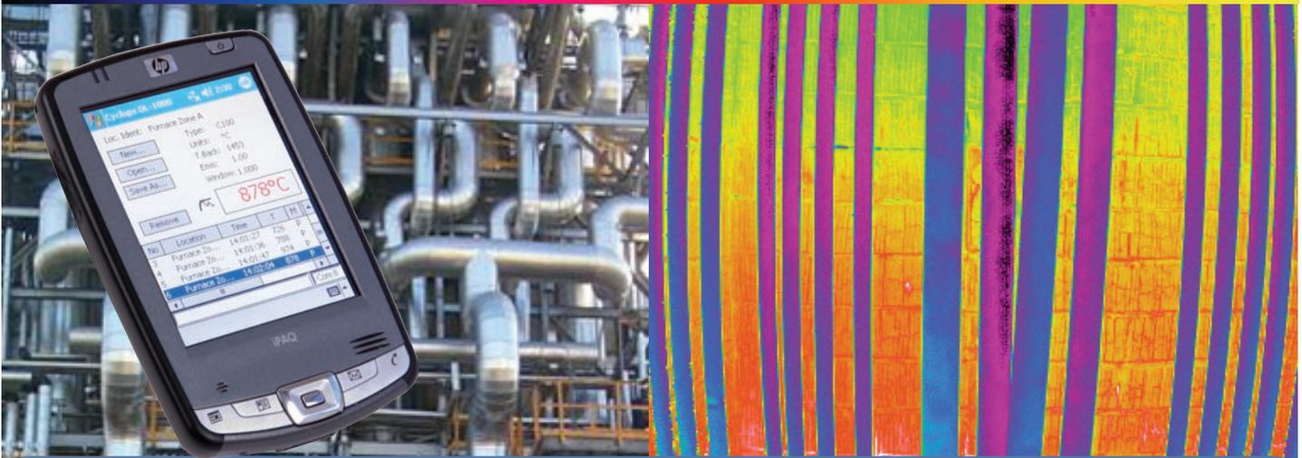
DL-1000 Data Logging System with Cyclops 390 FurnacePro for computing and logging true tube temperatures in pyrolysis, steam reforming furnaces and reheat furnaces in metals industries
