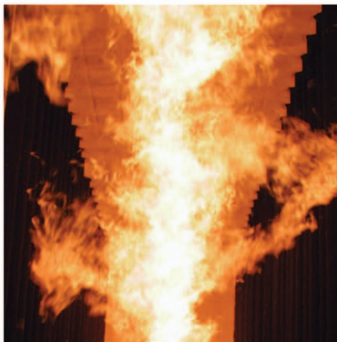
FIG. 5 Erratic flame pattern due to lack of oxygen.
