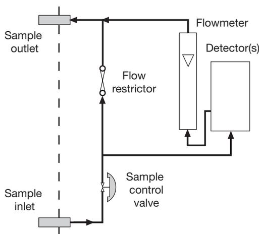
When the delays caused by lengthy external pipework are unacceptable, and there is sufficient sample available, the system illustrated here can be used.
