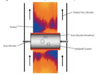
The HotSpotIR is easy to install, a quick release mounting bracket allows quick fitting and maintenance. The mounting bracket is keyed so that the exact same alignment is achieved when returning it to the mounting. A single, quick release cable connects the sensor to the alarm processor.
