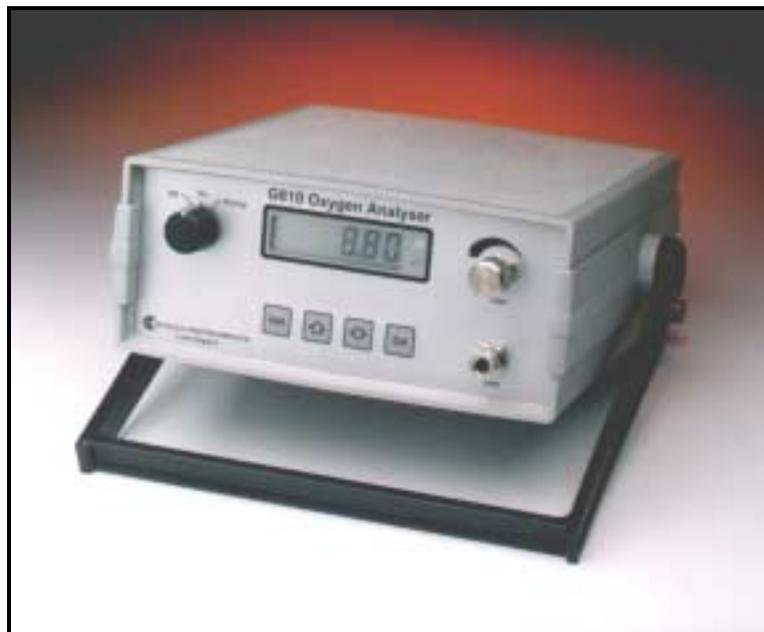
The **G810 oxygen analyser** is a portable instrument for measuring oxygen concentrations over a wide range. Based on a galvanic cell sensor, the analyser employs advanced linearisation to offer a high degree of accuracy whilst retaining the ability to be simply calibrated on air.
