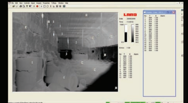
Point temperature measurement inside the furnace
