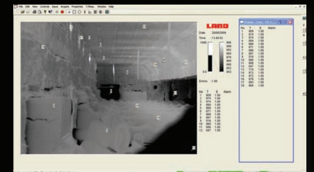
Point temperature measurement inside the furnace
