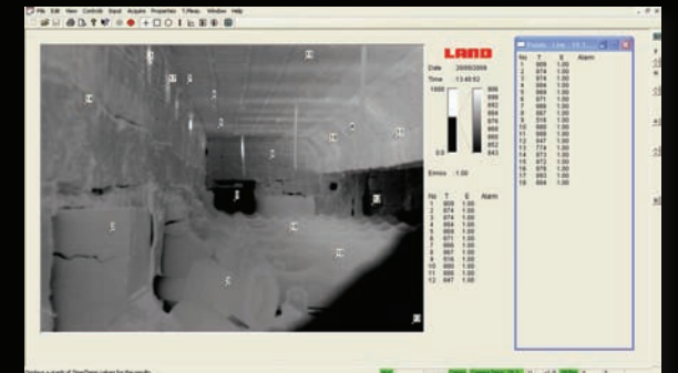
Point temperature measurement inside the furnace
