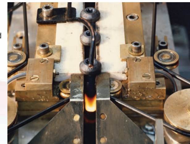
Induction heating application
