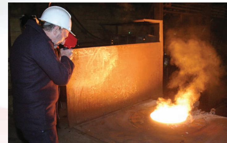
Accurate and repeatable readings can be taken from a safe distance throughout the plant
