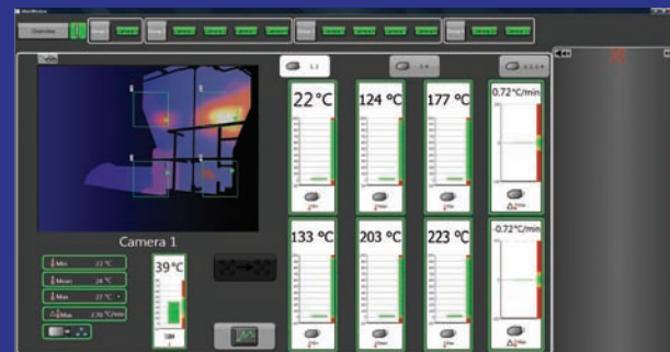
The individual camera display allows the operator access to detailed information from each measurement location.
