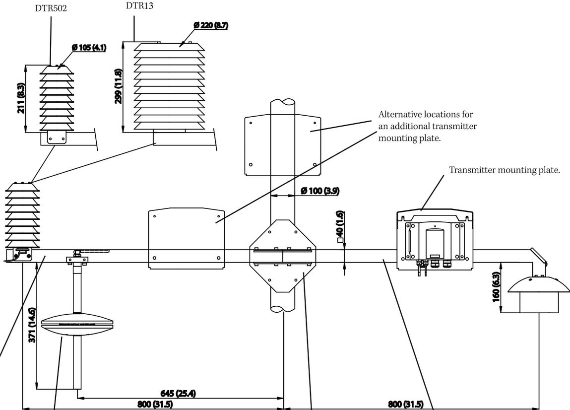
When Static pressure head (SPH10/20) is in use, the transmitter has to be installed to the pole mast. An airtight connection between the transmitter and the Static pressure head is made with a pressure hose. To prevent the condensed water from blocking the hose as it freezes, make sure that the hose won't hang loose.
